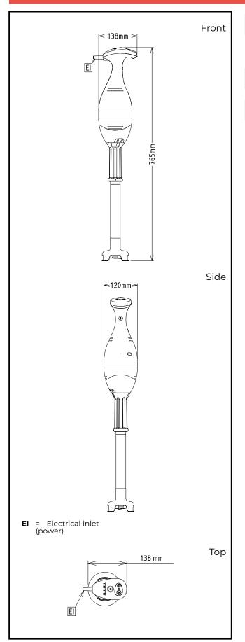
Electric Supply voltage: 220-240 V/1 ph/50/60 Hz **Electrical power max.:** 0.45 kW 0.45 kW **Total Watts:** Capacity: Capacity (up to): 100 Litre Key Information: External dimensions, Width: 138 mm External dimensions, 120 mm Depth: External dimensions, Height: 765 mm **Shipping weight:** 4.8 kg
